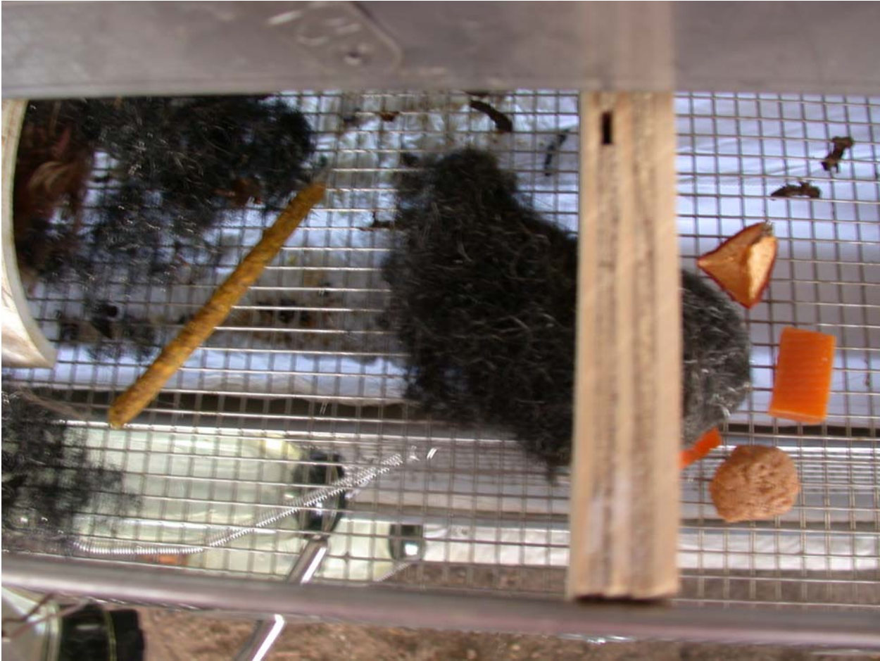
Figure 2. Maximum damage to a hole barrier by a rat.
