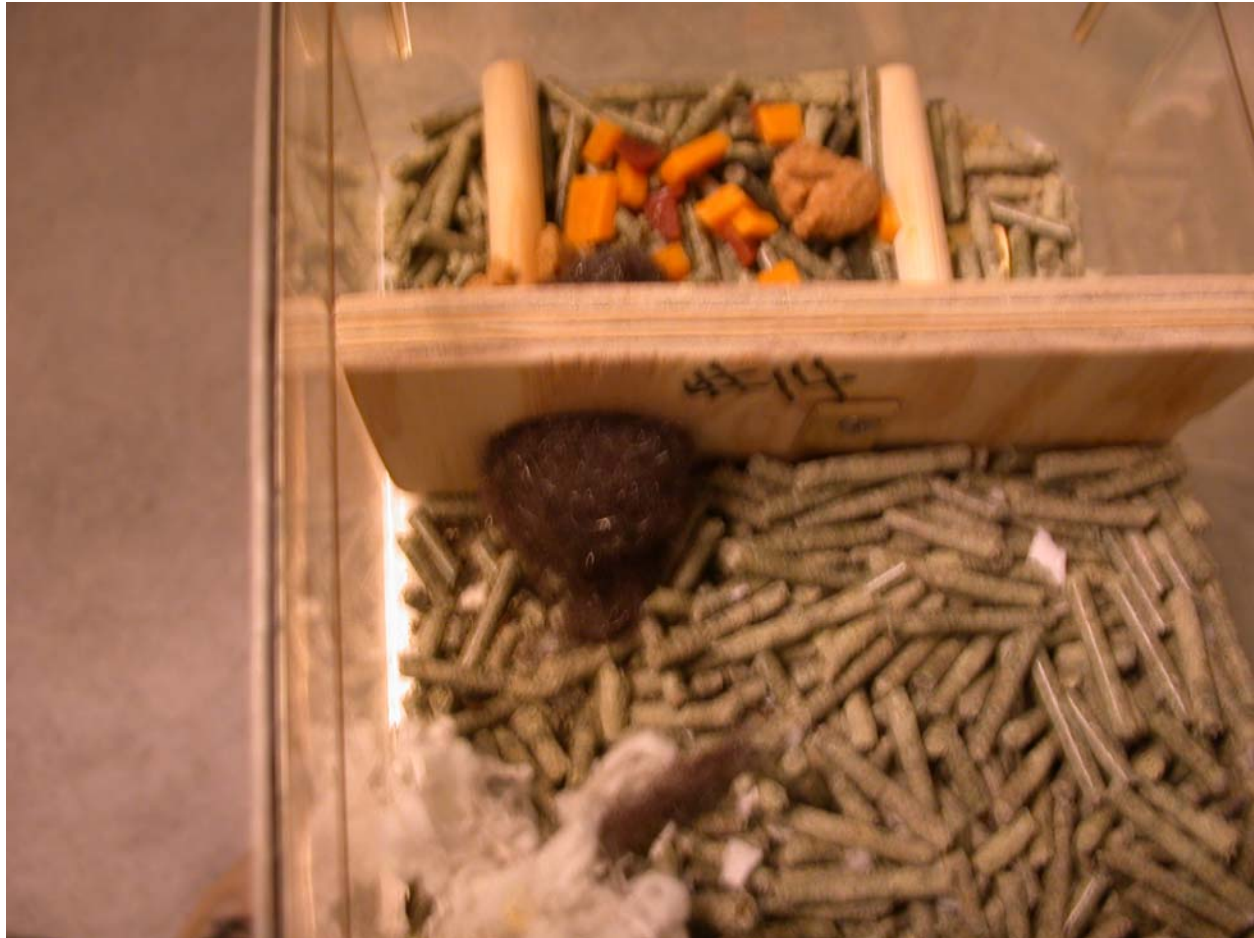
Figure 4. Maximum damage to a hole barrier by a house mouse.
